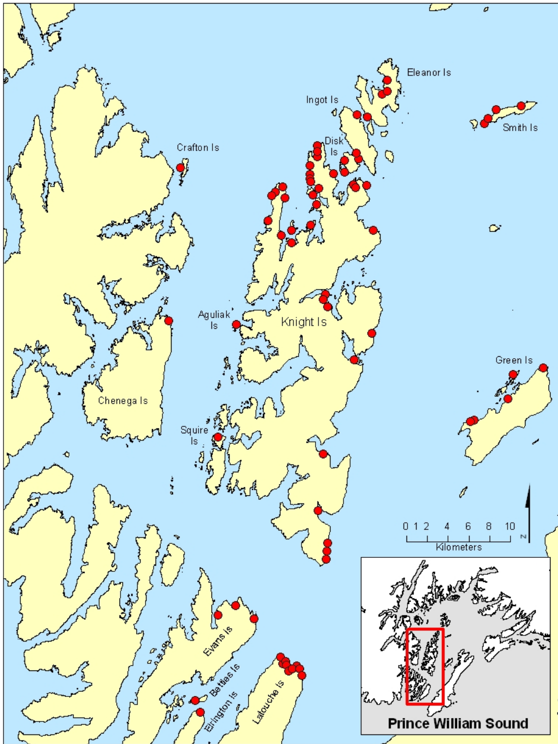
Figure 1. Map of the spill zone showing locations of all known surface and subsurface oil deposits. Filled red circles indication locations where subsurface oil has been found since 1998 (figure continued on following page).
